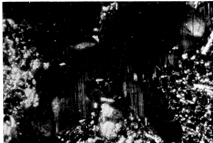
FIGURE 73. Leucite-bearing trachybasalt (351). Leucite occurring as the infilling of a small irregular cavity and displaying lamellar twinning. Crossed polars. (Magn. \times 135 .)
