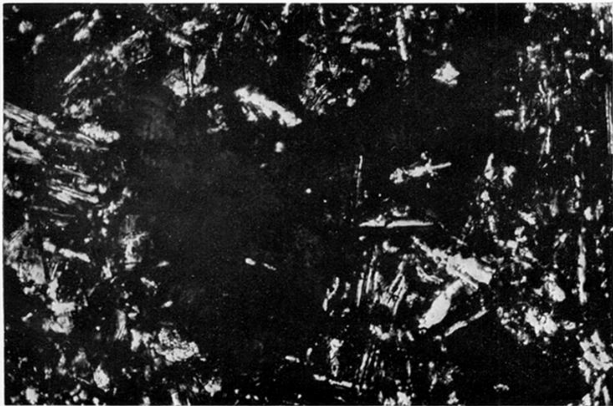
FIGURE 72. Leucite-bearing trachybasalt (351). Small plug 100 yards east of summit crater lake. Leucite occurring as a cavity infilling. Crossed polars. (Magn. \times 135 .)
