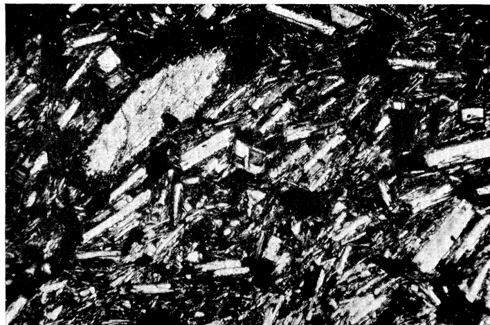
FIGURE 77. Trachyandesite (616). Central lava, 1961 Eruptive Centre. Phenocryst of amphibole in a groundmass of sub-parallel laths of zoned plagioclase An_{58} to An_{40} , pyroxene and iron ore. Crossed polars. (Magn. \times 34 .)
