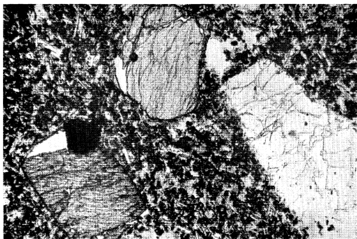
FIGURE 68. Ankaramite (114). Base of Main Cliffs east end of Sandy Point. Phenocrysts of olivine, pyroxene and plagioclase set in a groundmass of pyroxene, plagioclase and iron ore. Plane polarized light. (Magn. \times 34 .)
